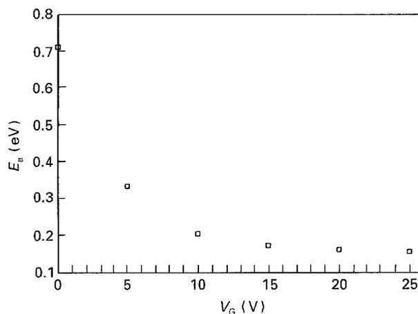
Figure 7 The activation energy,  $E_a$ , of a-Si:H TFTs as a function of the gate voltage,  $V_G$ .
