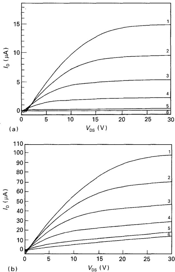
Figure 2 (a) The TFT drain to source current,  $I_D$  versus the drain to source voltage,  $V_{DS}$ , at 304 K for various gate voltages,  $V_G$ . (b) The TFT drain to source current,  $I_D$ , versus the drain to source voltage,  $V_{DS}$  at 444 K for various gate voltages,  $V_G$ . Values of  $V_G$  for curves 1–6: 0, 5, 10, 15, 20, and 25 V.
