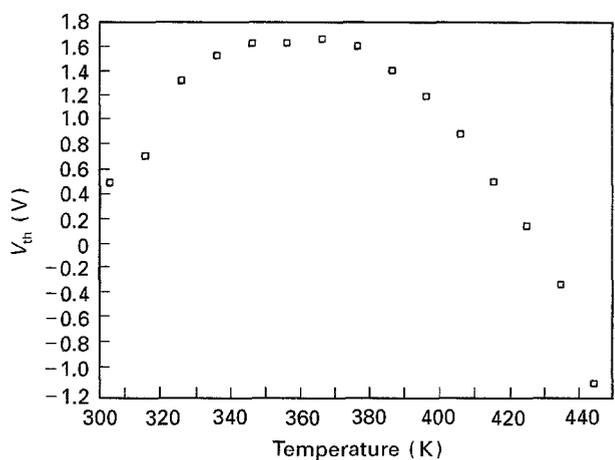
Figure 4 The threshold voltage,  $V_{th}$ , of a-Si:H TFTs at ambient temperatures from 300–450 K.
