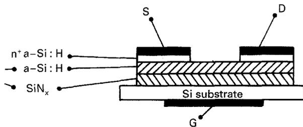
Figure 1 Structure of amorphous silicon thin-film transistors (a-Si TFT). S, source; D, drain; G, gate.
