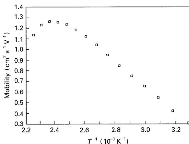
Figure 6 The field-effect mobility versus inverse temperature for ambient temperatures from 300–450 K.
