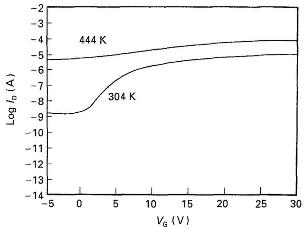
Figure 3 The transfer characteristics of a-Si:H TFTs at ambient temperatures 304 and 444 K.
