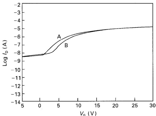
Figure 5 The measured transfer characteristics of the a-Si:H TFT at 314 K. Curve A was obtained for the sample kept at 314 K, while the curve B was obtained after the sample had been subjected to a heating cycle from 314–444 K, and then cooled to 314 K.
